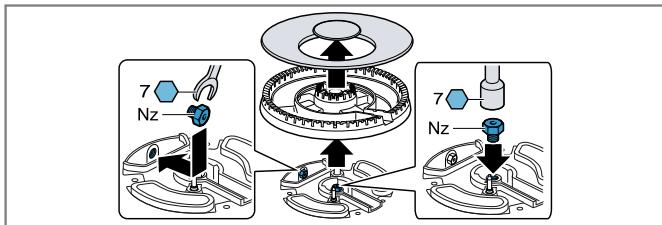
Ensure that the nozzle does not become detached during removal or fastening.
