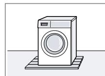
Place the appliance on a water-resistant wooden board (minimum thickness of 30 mm) which is screwed tightly to the floor.
